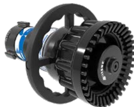
M-R1000-NJ — 2.5"NH Automatic Pressure Nozzle 150-1000 gpm flow range (600-4000 l/min) @ 100 psi
